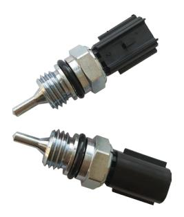
The Coolant Temperature Sensor (CTS) monitors the temperature of the coolant that is being pumped around the battery to cool the battery module of EV/PHEVs. If the battery module starts to overheat, the Coolant Temperature Sensor relays a signal to the Battery Management System (BMS). The BMS uses this information to prevent battery packs from any damage and maximize the performance.
