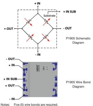
Both +IN and +IN SUB need to be connected to the highest potential in the circuitry.
